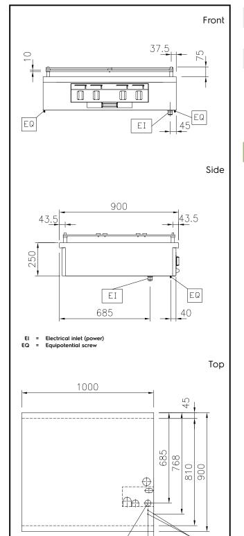
Electric Supply voltage: 440 V/3 ph/50/60 Hz Total Watts: 16 kW **Key Information: Working Temperature MIN:** 80 °C **Working Temperature MAX:** 350 °C 1000 mm External dimensions, Width: External dimensions, Depth: 900 mm External dimensions, Height: 250 mm Net weight: 160 kg Configuration: One-Side Operated;Top Sustainability
